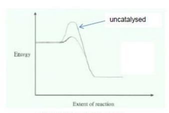
exothermic profile drawn (1) uncatalysed / catalysed line labelled (1)
